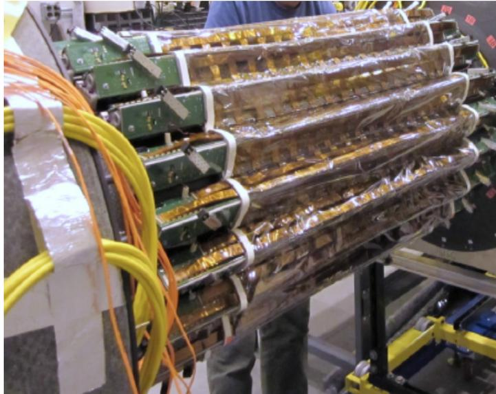
**Figure 2.6: Picture of the SSD assembled and mounted on its support structure.**
