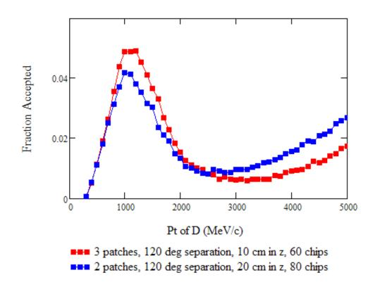
Fig. 5 Geometrical efficiency comparing a 3 patch configuration with a 2 patch configuration. The two patch example in this case has longer active ladders and requires more chips (80 chips) than the 3 patch configuration (60 chips). Even with fewer chips the 3 patch pattern one gets better performance in the 1 GeV Pt region.
