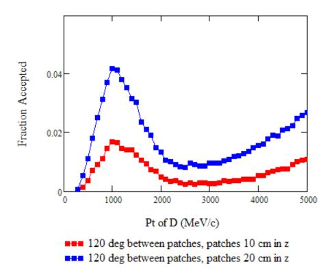
Fig. 4 Geometrical efficiency for two patches of detector shown as a function of D Pt. Two cases are shown with different patch lengths, 10 and 20 cm long in z. The two patches are separated by 120 degrees. The 10 cm configuration requires 40 detector chips and the 20 cm configuration would require 80 chips.
