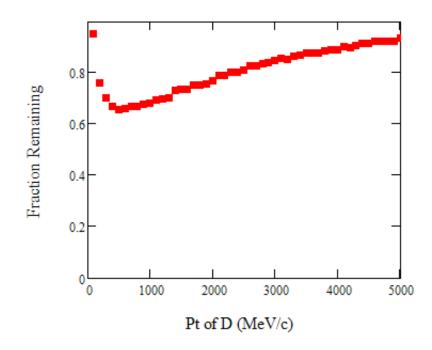
Fig. 1 Fraction of pairs remaining after requiring that both the pion and kaon have a momentum greater than 800 MeV/c shown as a function of D pt. This shows that not too many pairs are rejected using this momentum constraint.
