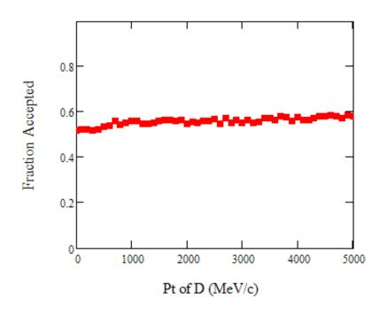
Fig. 2 Geometrical efficiency for detecting both the K and the p in a 20 cm long cylinder with an
