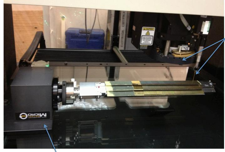
vision and stylus probes, both with µm level precision
