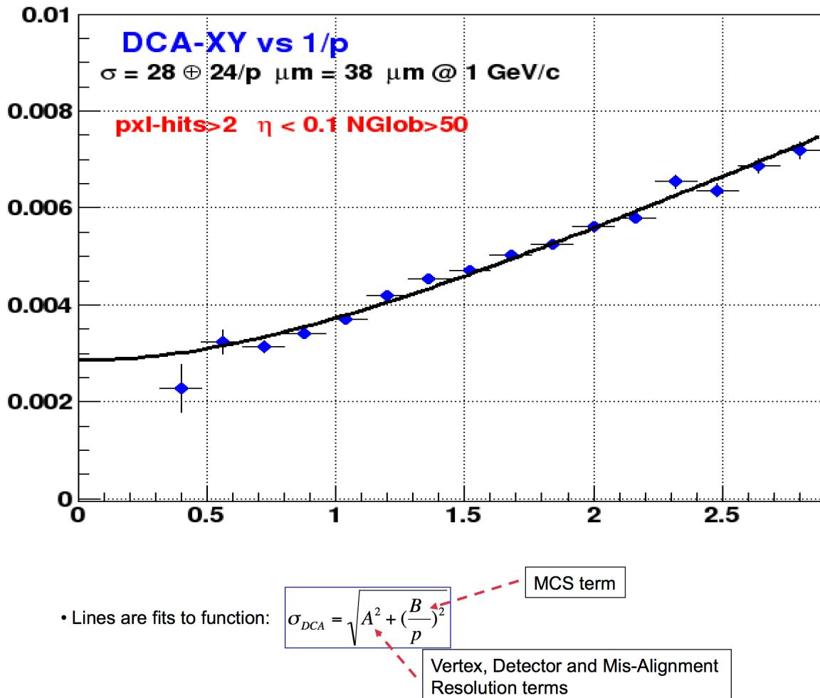
*Figure 2 : Preliminary pointing resolution of the HFT detector in the transverse plane (X-Y).*
