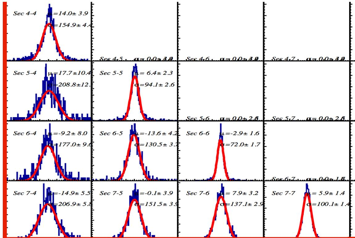
*Figure 1 : Example of PXL Sector-to-Sector alignment verification and fine tuning using a low luminosity, magnet off, data sample. The figure shows the difference in the X-coordinate of the event vertex reconstructed from tracks passing through two different Pxl sectors (off diagonal elements) or a sector and the full detector (diagonal elements). We observe relative deviations around 10 microns.*
