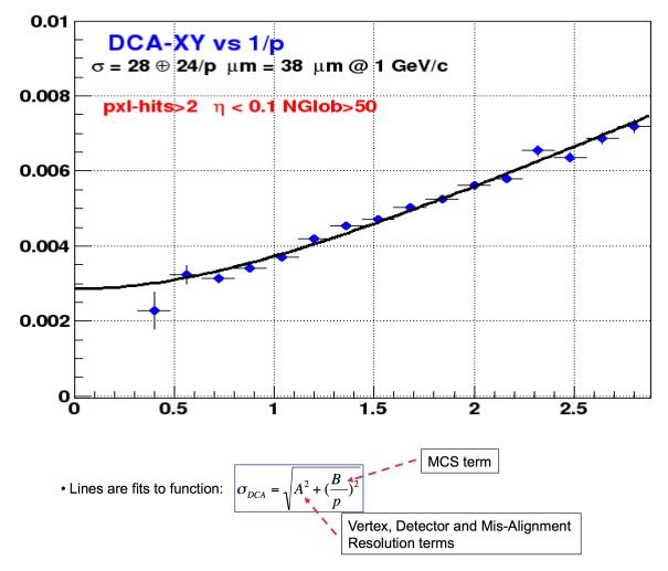
Figure 1 : Preliminary pointing resolution of the HFT detector in the transverse plane (X-Y).
