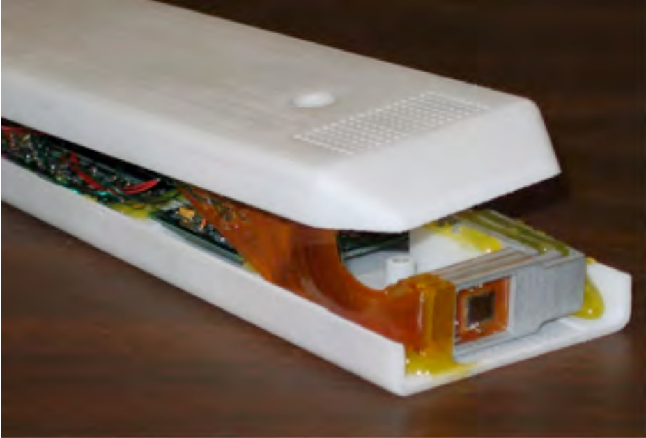
Figure 29: Three Mimosrat-2 sensors in a telescope configuration used in a beam, test at STAR.
