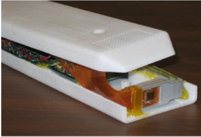
Figure 27: Three Mimostar-2 sensors in a telescope configuration used in a beam, test at STAR.
