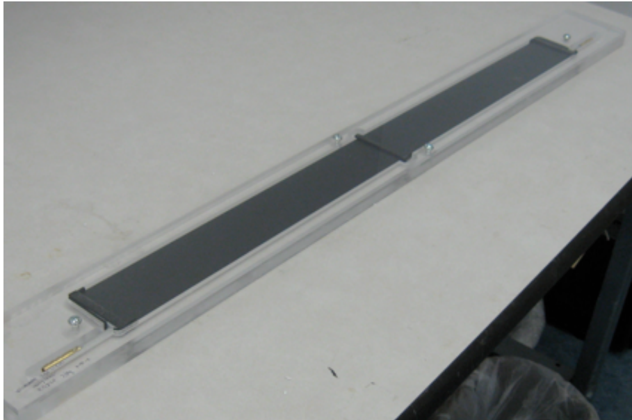
Figure 50: Long IST prototype ladder made out of carbon fiber honeycomb and carbon fiber skins. This prototype has one cooling channel.
