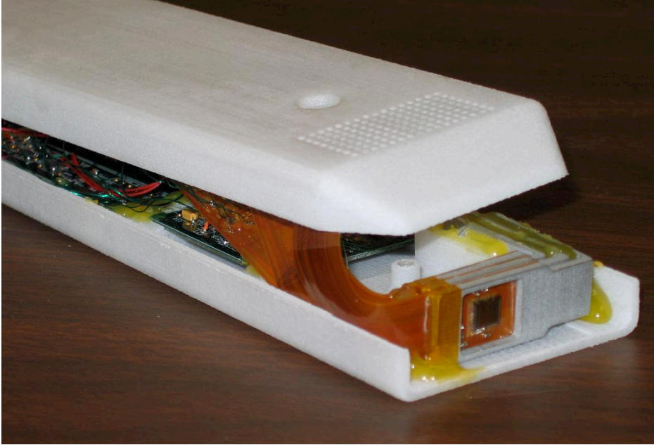
Figure 14: Three Mimostar-2 sensors in a telescope configuration used in a beam, test at STAR.
