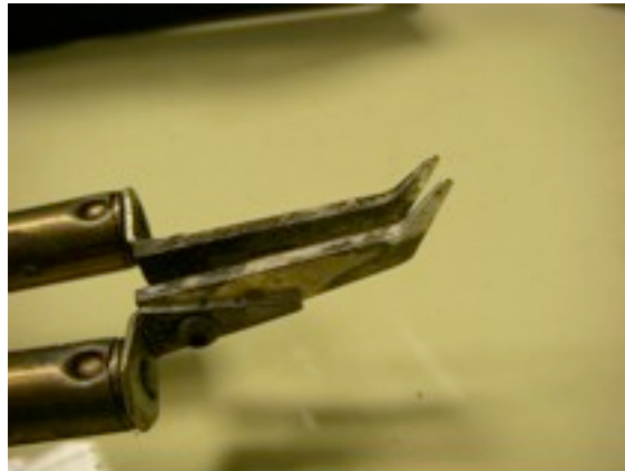
Figure 53: This soldering head will be used to remove the leaking capacitors on some ladders.
