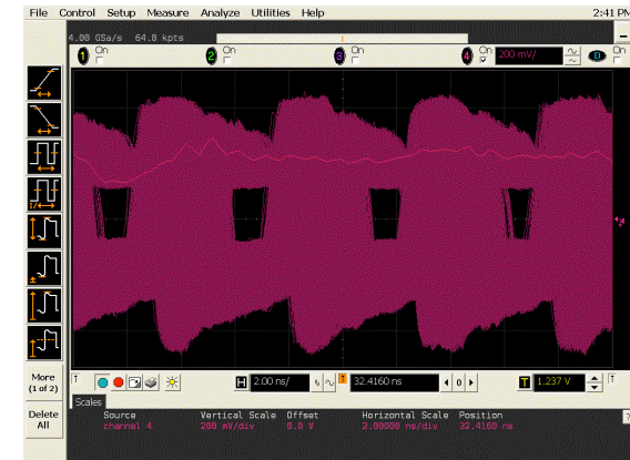
Un-buffered path 200 MHz 1.0 m cables
