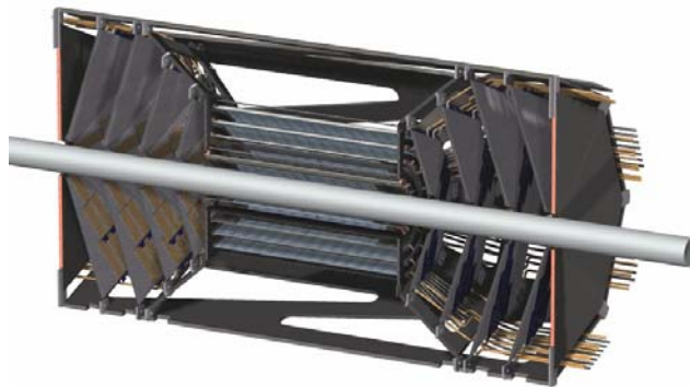
Figure 2. A schematic cut-away mechanical drawing of the proposed vertex detector (from Hytec).
