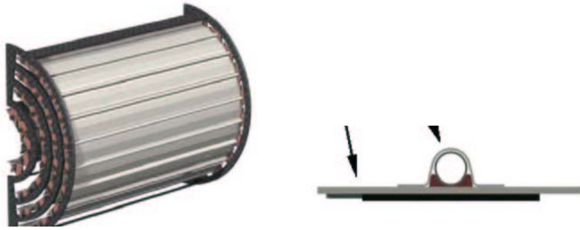
Figure 65 3D model of the barrel region on the left and the ladder structure on the right showing a cooling tube mounted on a C-C thermal plane and the sensor and electronics on the underside.
