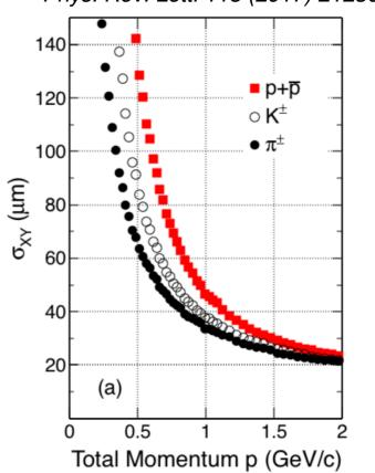
STAR Heavy Flavor Tracker (HFT) provides excellent vertex/track-dca resolution and allows reconstruction of charm hadron decays
