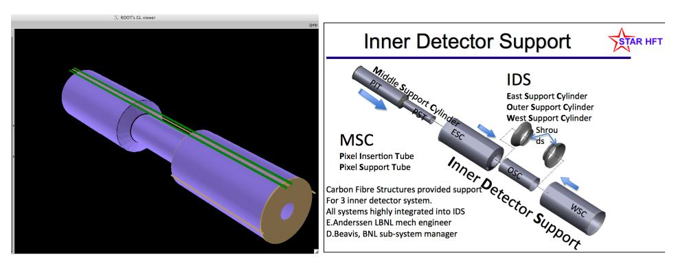
Plot of "IDSM" volume done using agml geometry
