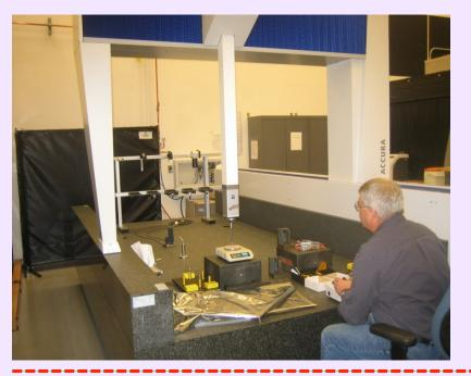
ZEISS: touch probe 2-3  $\mu$ m (xyz) and visual 2-3  $\mu$ m (xy) 50  $\mu$ m (z)
