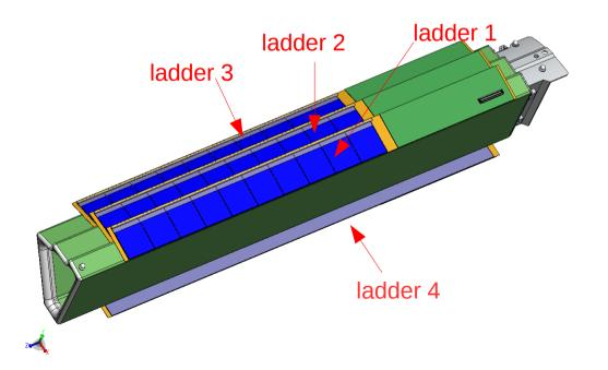
overlap  $\rightarrow$  ladders 2 and 3 need to be (partially) surveyed with the touch probe
