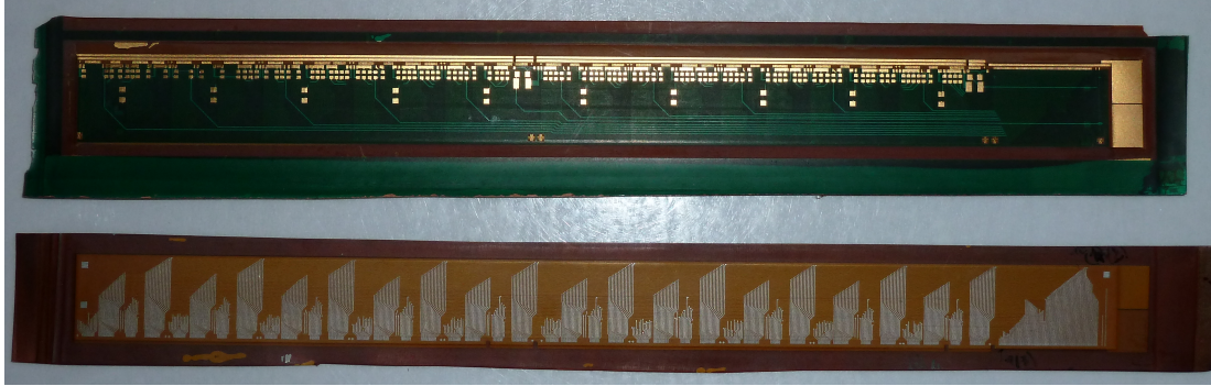
Figure 1 Aluminum conductor flex cable developed for the ALICE PXL detector. This cable is four layers with micro-vias and a 50 um feature size. The top side of the cable is gold plated to allow for wire-bonding and soldering. The lower cable in the picture shows one of the inner layers in aluminum conductor.
