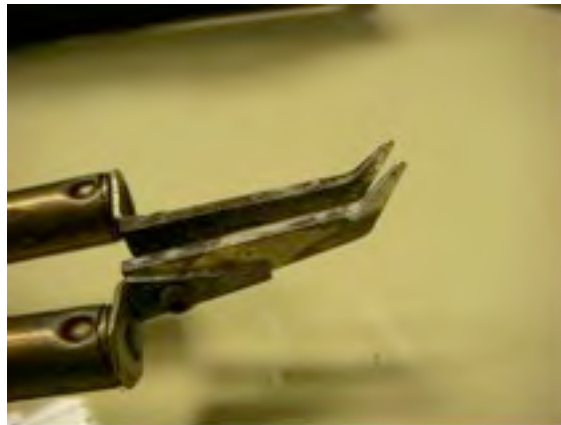
Figure 66: This soldering head will be used to remove the leaking capacitors on some ladders.
