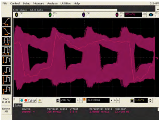
Buffered path 200 MHz 1.0 m cables
