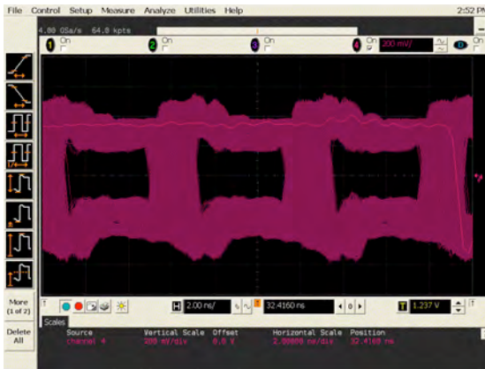
Buffered path 160 MHz 1.0 m cables
