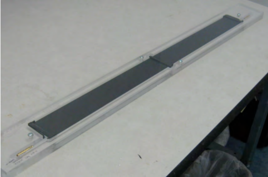
Figure 51: Long IST prototype ladder made out of carbon fiber honeycomb and carbon fiber skins. This prototype has one cooling channel.
