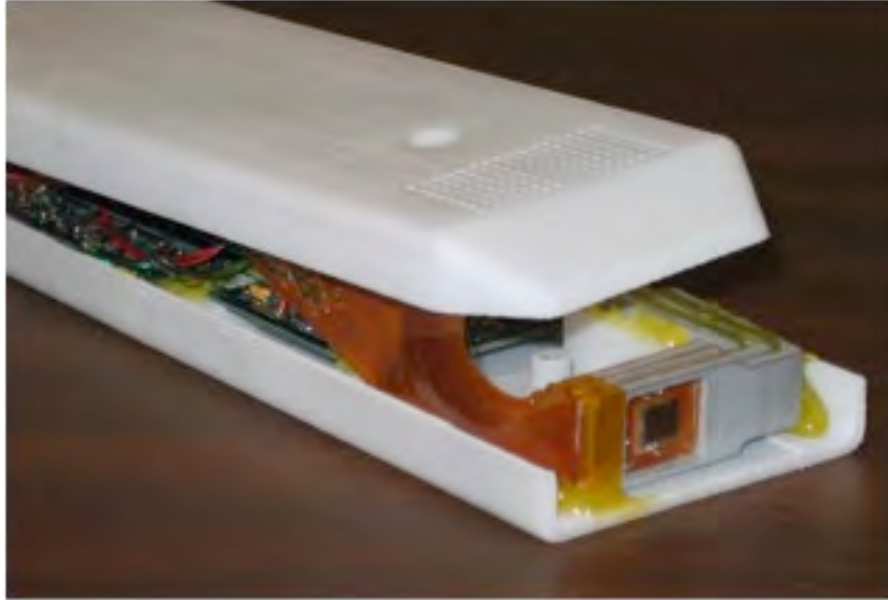
Figure 28: Three Mimostar-2 sensors in a telescope configuration used in a beam, test at STAR.
