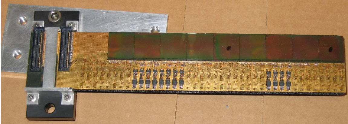
Figure 66: A prototype ladder showing low mass PCB, MIMOSA5 detectors and driver electronics bonded to a mechanical carbon fiber and reticulated vitreous carbon foam based carrier.
