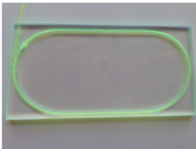
Figure C.5.1: One of 12cm \times 5.5cm \times 0.5cm EJ-200 scintillator with a triple layer of Kuraray Y-11 WLS fibers glued with EJ-500 optical cement
