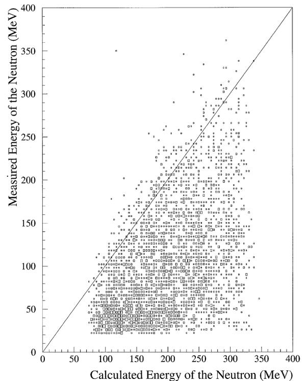
Fig. 10. The neutron detected energy is plotted versus the calculated neutron energy computed from the two-body kinematics for the CEX reaction. A general energy inefficiency is evident and is discussed in the text.
