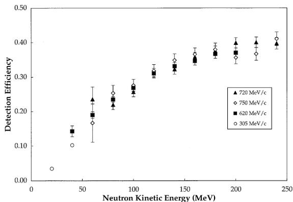
Fig. 8. The neutron detection efficiency obtained from the four data sets at four momenta are shown to illustrate the internal consistency of our analysis.
