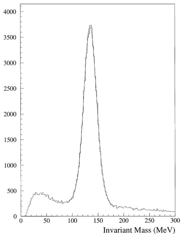
Fig. 2. The invariant mass of all two-photon clusters shows clear evidence for a  $\pi^0$  mass peak on a continuous background. A Gaussian fit to the  $\pi^0$  mass peak gives a FWHM of 29.4 MeV and a centroid of 134.6 MeV.
