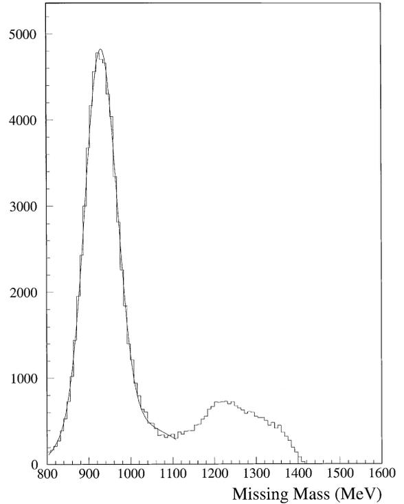
Fig. 4. The missing mass for the reaction  $\pi^-p \rightarrow \pi^0 X$  is shown here for all events from Fig. 2 whose  $\pi^0$  invariant mass was in the range 110–160 MeV. Events in the peak within  $\pm 50$  MeV of the neutron mass were deemed to be consistent with the CEX reaction  $\pi^-p \rightarrow \pi^0 n$  and were therefore included in our sample for neutron studies in the Crystal Ball.
