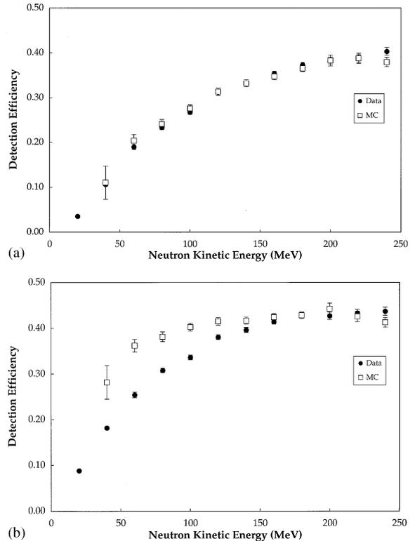
Fig. 7. (a) The neutron detection efficiency obtained from data and from Monte Carlo is displayed as a function of the neutron energy incident on the NaI, with a 20 MeV cluster energy threshold used in the analysis. The Monte Carlo events were simulated using the FLUKA/GHEISHA codes in GEANT. The neutral-hadron cutoff was set to 2 MeV in the Monte Carlo. (b) The same plot as in Fig. 7a except that a 10 MeV cluster energy threshold was used in the analysis.
