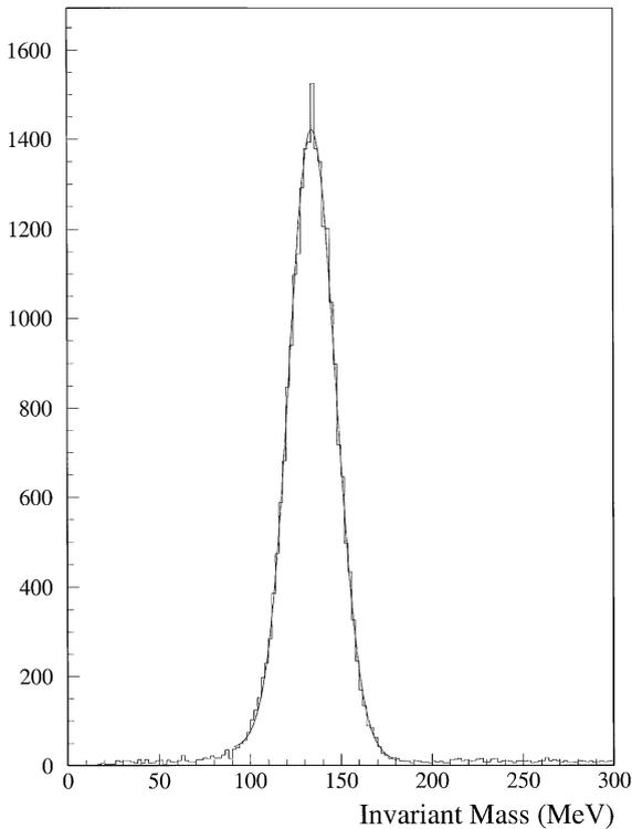
Fig. 3. The invariant mass of two-photon clusters simulated in the GEANT-based Monte Carlo. The FWHM of the  $\pi^0$  mass peak is 29.2 MeV with the centroid at 134.7 MeV, in good agreement with the fitted results shown in Fig. 2.
