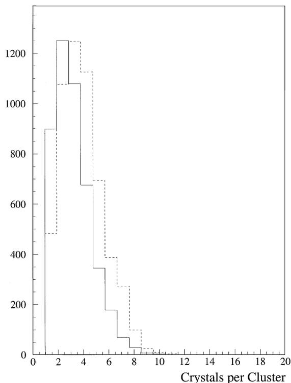
Fig. 11. We show the crystal multiplicity per cluster for neutron-induced events as measured in our CEX data as the solid line, and as simulated CEX events in the GEANT Monte Carlo with the FLUKA/GHEISHA neutron simulation codes as the dashed line. There is a systematic shift of one crystal per cluster on average placing the Monte Carlo multiplicities higher than those from the data. Moreover, the agreement depends on the choice of the neutral-hadron cutoff energy.
