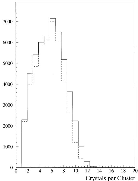
Fig. 9. The multiplicity distribution of crystals per cluster is given for photon interactions in NaI as measured with CEX events in our data. For comparison, the same quantity is shown for the GEANT simulation of photon interactions from CEX events as the dashed line. The agreement is a good one.
