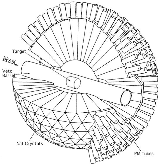
Fig. 1. A diagrammatic representation of the CB is shown along with the veto barrel and the target. (The target is located inside the veto barrel.) The veto barrel is segmented into four sections along the cylinder axis with each section read out by photomultiplier tubes at both ends.
