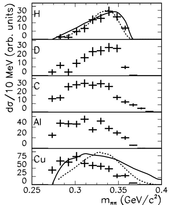
FIG. 3. Experimental results for the  $2\pi^0$  invariant mass distributions obtained for the H, D, C, Al, and Cu targets corrected for Crystal Ball acceptance. The vertical scale is in arbitrary units. The solid lines show the results of calculations made by Rapp [18], and the dashed line is the prediction by Vicente Vacas [16].
