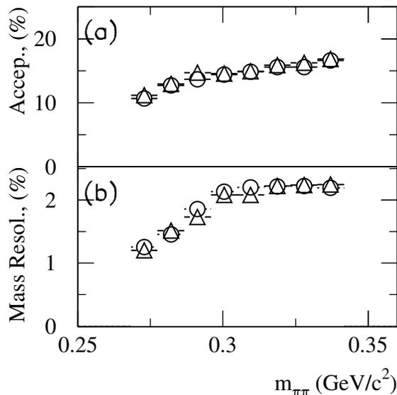
FIG. 1. (a) The  $2\pi^0$  acceptance at 0.408 GeV/c as a function of the  $2\pi^0$  invariant mass  $m_{\pi^0\pi^0}$ , calculated by a Monte Carlo simulation. (b) Invariant-mass resolution of the CB detector at 0.408 GeV/c calculated by using Monte Carlo. The triangles show the values for the hydrogen target, the circles for the carbon target.
