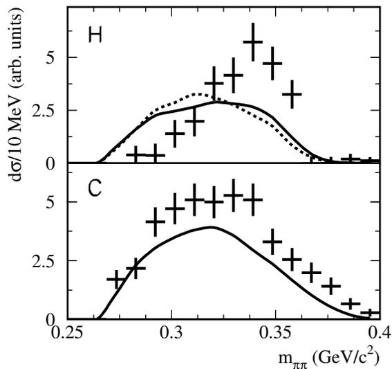
FIG. 2. Experiments results for the  $2\pi^0$  invariant mass distributions (crosses) for H and C targets uncorrected for acceptance. The solid line is the Monte Carlo calculated  $m_{\pi^0\pi^0}$  assuming pure phase space; see text for details. The dashed line is the spectrum based on a Monte Carlo calculation of the sequential process  $\pi^- p \rightarrow \Delta^0 \pi^0 \rightarrow \pi^0 \pi^0 n$ .
