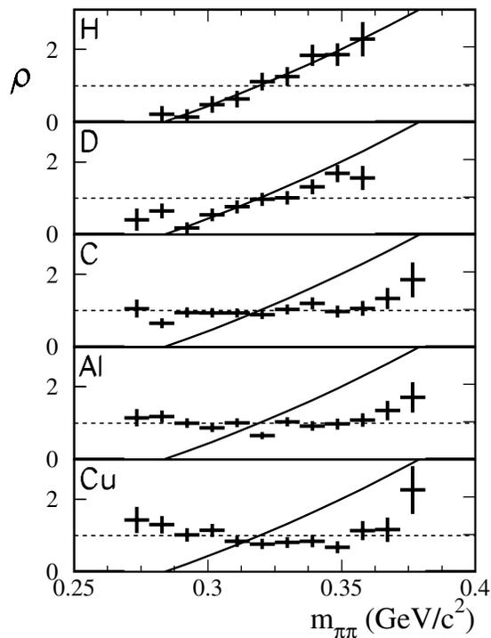
FIG. 4. Illustration of the change in the  $\pi^0\pi^0$  invariant mass spectrum as expressed by the ratio  $\rho = m_{\pi\pi}(\text{data})/m_{\pi\pi}(\text{phase space})$ . The ratio is calculated for each of our five targets. The solid line is a second-order polynomial fit to the data on H. The dashed line represents  $\rho = 1$ .
